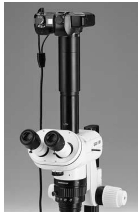
2.5× projection eyepiece, T2 camera adapter, Ricoh XR-X3000D single-lens reflex camera and remote-release key
