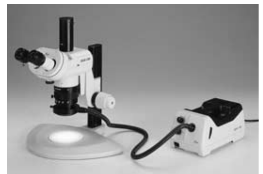
Leica M420 with cold-light source Leica CLS150 and ring lamp
