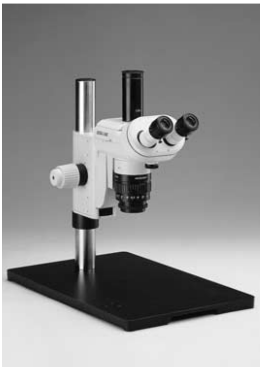
Drive housing with coarse/fine drive on universal stand
