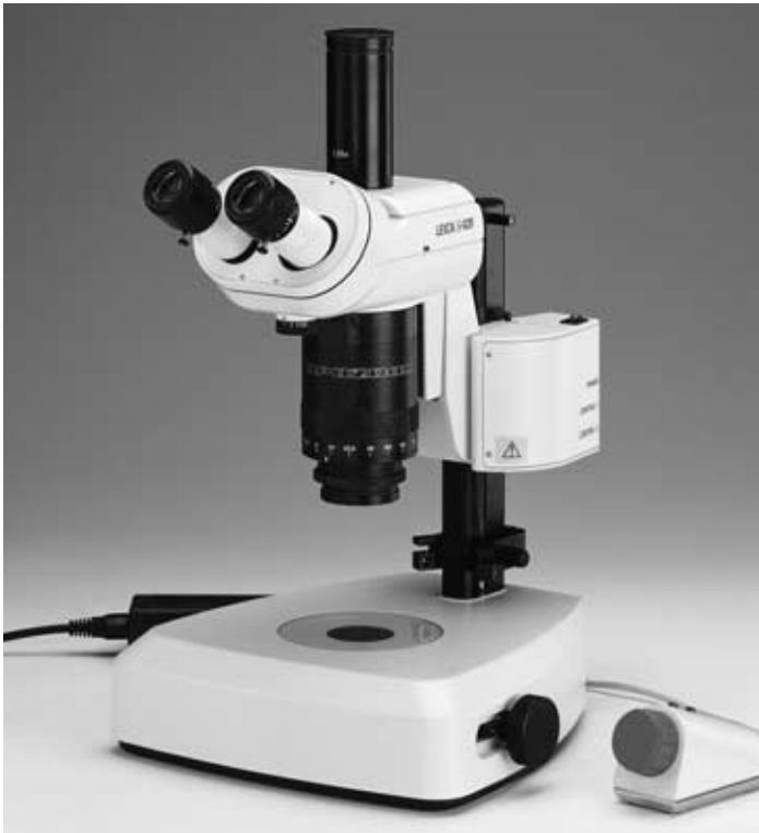
Motor-focus system, on transmitted-light stand HL
