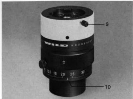
Loosen the clamping screw (9) of the Macrozoom objective and insert the latter in the dovetail ring beneath the optics carrier (4) so that the index mark (10) of the magnification scale points towards the user. Tighten the clamping screw (9) securely.
