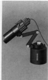
The lampholder (11) can be fitted to the adapter (12) of the incident-light base. Loosen screw (21), fit the low-voltage lamp, and retighten screw (21). To align the lamp with the specimen, the lampholder can be turned on the adapter (12), tilted by means of the articulated arm, and swung sideways on the lampholder.
